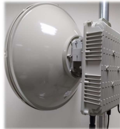
Dual-channels in each subband using dual polarization (XPIC) with OMT
